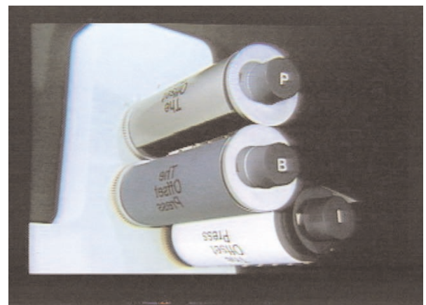
A model of a three-cylinder offset-lithographic press.
